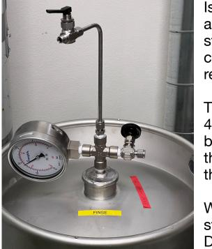
Isotope water standard waters are filtered and stored in 50L stainless steel beverage containers, following IAEA recommendations.
