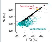
Condensation issues. Turning off the counterflow at altitude reveals the extent of possible condensation problems: d-excess takes minutes to reset.
